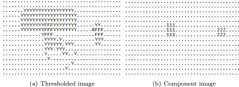
Figure 1: An example thresholded image is shown in (a), with “Y” representing pixels corresponding to the yellow goal and “F” representing pixels corresponding to food. The goal pixels that appear below the ninth row from the bottom are noise. Goal noise is avoided by only searching the top four lines for the goal. The corresponding food component image is shown in (b), clearly segmenting the two foods into component 1 and component 2, so that a distance and angle can be calculated to each.
